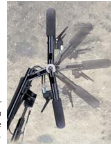
Adjustable-angle stroller handles provide maximum flexibility in adjusting the chair's geometry.
