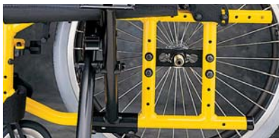
The Allegro's unique modular crossbrace system allows a host of configuration possibilities.
