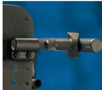
Newly designed adjustable angle footplate provides a positive lock for dorsi or planar flexion.
