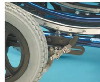
Redesigned bolt-on wheel locks can be used with any wheel selection and can be switched from a push-to-lock to a pull-to-lock configuration in seconds.
