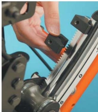
Redesigned tilt lock-out stops may be used to limit the tilt range on the low end, high end or both.
