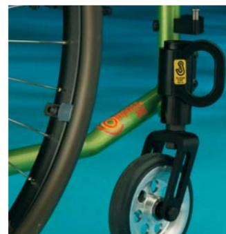
Front transport tie-down brackets are clearly marked.\*
