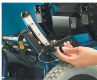
Rear tie-down brackets and locking pins are easily accessible to caregivers.
