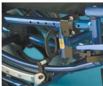
Front tie-down brackets are attached to seat frame and clearly marked.
