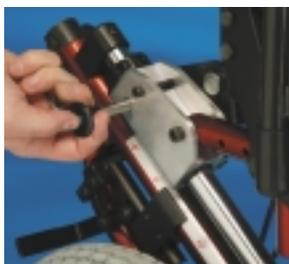
Transport locking pins should be used to lock gear rack when chair is transported by bus or van.\*
