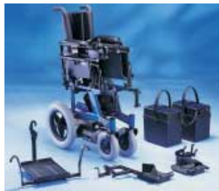
The R51, R51LX and R51LXP can be disassembled and folded for easy transport.
