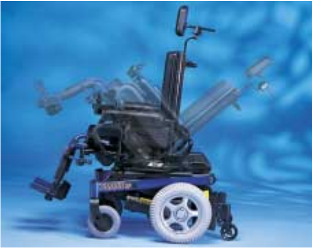
As the Invacare 2GT tilts from 0° to 50°, the system shifts along the base and optional active anti-tippers are extended to help maintain stability.
