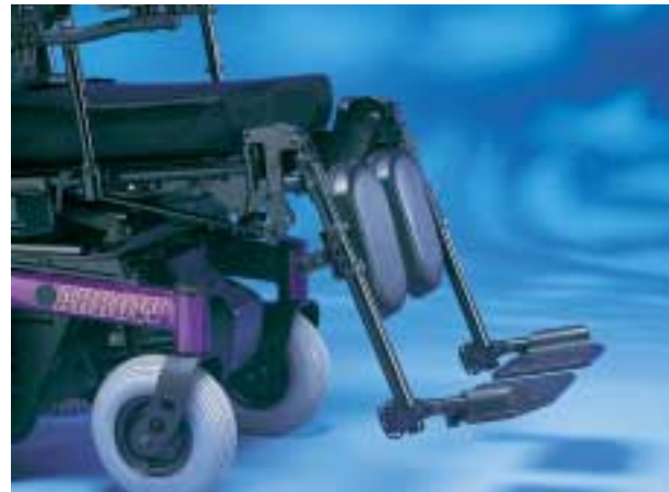
Standard on the 2GTR is the mechanically elevating legrest system, which consists of two push rods acting with the recline motion to elevate the legrests. The system will interface with either the Genius articulating/elevating legrests or the AT5544 basic elevating legrests. To elevate the legrests without reclining, upgrade to the power-elevating legrests.
