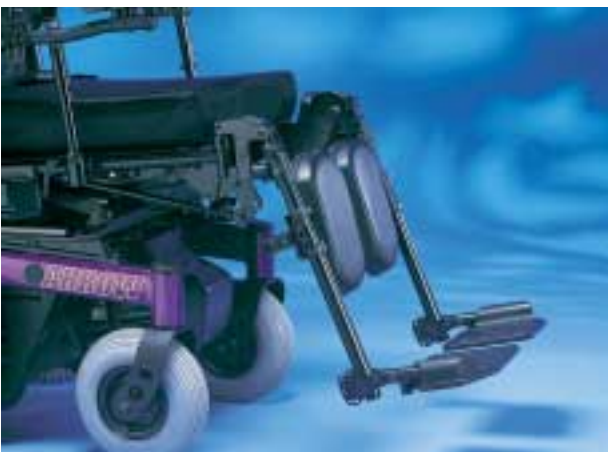
Standard on the 2GR is the mechanically elevating legrest system, which consists of two push rods acting with the recline motion to elevate the legrests. This system interfaces with either the Genius articulating/elevating legrests or the AT5544 basic elevating legrests. To elevate the legrests without reclining, upgrade to the power-elevating legrests.
