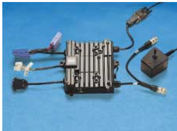
Standard on the 2GTR, the TRCM (Tilt Recline Control Module) provides control of any combination of five actuators through a variety of options: 1) Through-the-driver control – Accomplished through programming of the MKIV, with no additional components. 2) 4-way toggle – Provides consumer control or can act as an attendant control. The TRCM can be programmed to limit the tilt/recline range, drive lockout, acceleration, deceleration and actuator speed.
