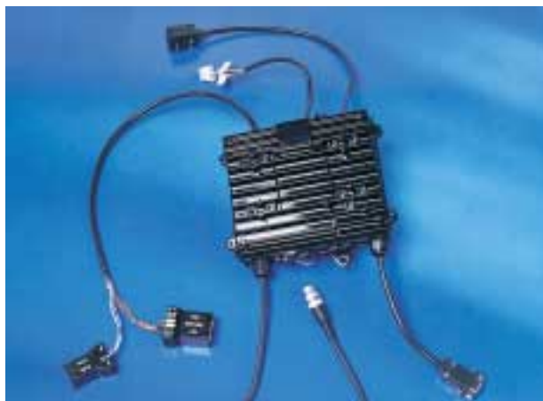
Standard on the 2GR, the TAC (two-actuator control) provides control of any combination of two actuators through a variety of options: 1) Through-the-driver control – accomplished through programming of the MKIV™ with no additional components. 2) 4-way toggle – provides user control or can act as an attendant control. 3) Any two ability switches – can be plugged into the mono jacks on the TAC to control the actuators. The TAC also can be programmed to limit the tilt/recline range, drive lockout, acceleration, deceleration and actuator speed.
