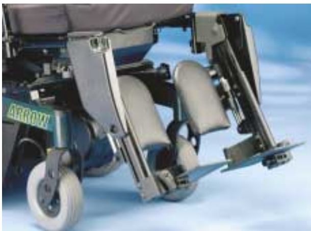
Power-elevating legrests are available as an option on the 2GT, 2GR and 2GTR, featuring anti-rotational footplate design, actuator built into the legrests, low-profile mounting, easy swing-away and disconnect.
