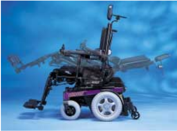
As the Invacare 2GTR tilts from 0° to 50° and reclines from 90° to 175°, the system shifts along the base and optional active anti-tippers are extended to help maintain stability.
