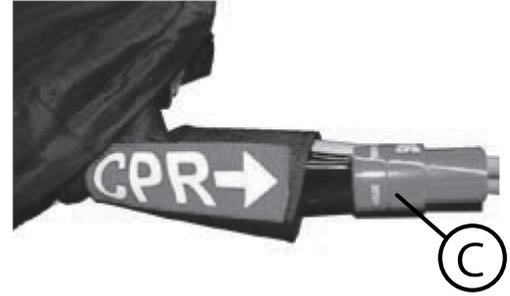
3. Disconnect the red CPR connector Ⓒ located on the hose.
