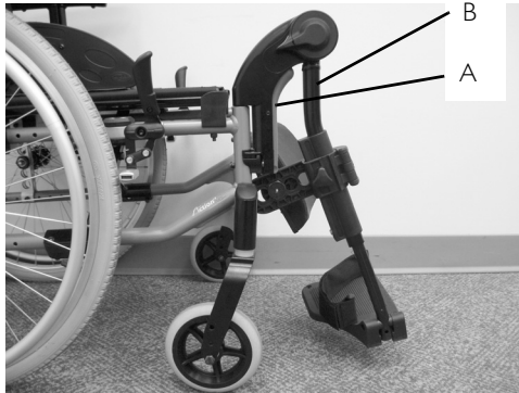
FIGURE 17 Installing/Removing Elevating Legrests - MyOn and MyOn Active - Removing
