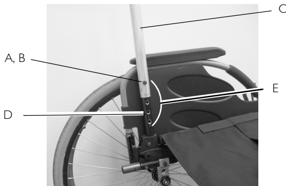
FIGURE 5 Adjusting the Height Adjustable Back
